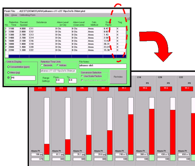
Figure 11- Virtual chemical sensors created from a list of compound retention times.
